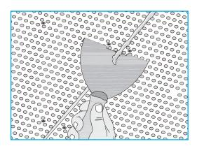
FIGURE 10 'Chipping' Off Excess Filler
