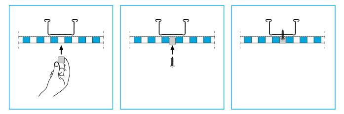
FIGURE 7 Cap Installation
