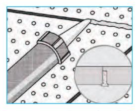
FIGURE 9 Joint Filling (with Uniflott)
