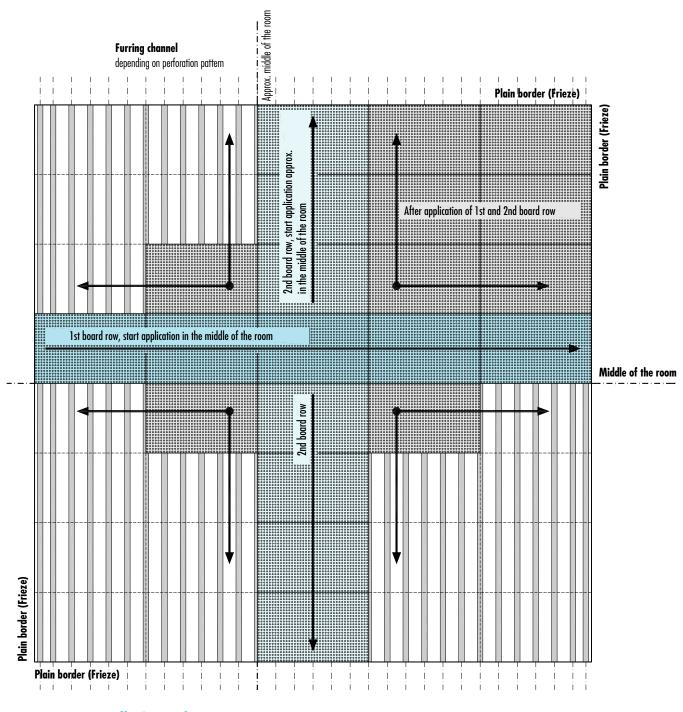
**FIGURE 3 Installation Scheme**
