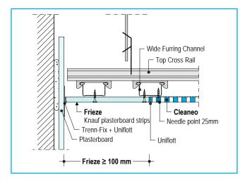
FIGURE 16 Connection to Wall
