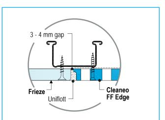
FIGURE 19 Connection to Frieze with Cleaneo FF Edge
