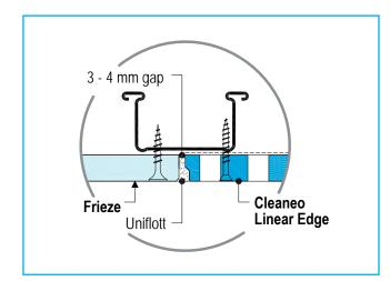
FIGURE 18 Connection to Frieze with Cleaneo Linear Edge
